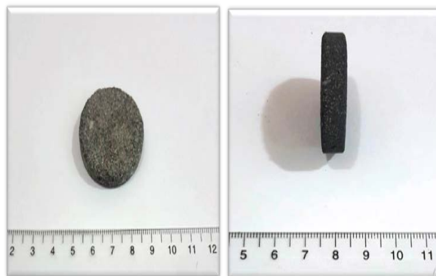
Fig. 2 Sample of (R-Ce) represent it's Diameter and Thickness.
